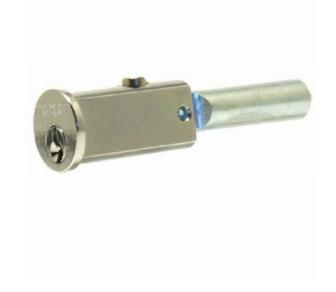
Extruded brass body, bright chrome plated Body size 22mm diameter x 14mm across flats, 46mm length Face dimensions 25mm diameter x 3mm Hardened steel bullet, 12.5mm diameter x 50mm length Supplied with 2 numbered keys
